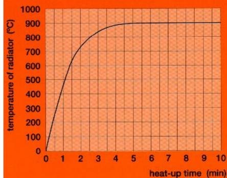
3 Heat-up curve of Elstein SHTS Super High Temperature Radiators
